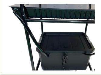
5. -- **SGO-36**: Place the shorter frame with the *B2* legs to the left of the frame with the reservoir. Connect the two trays with the 6" section of tubing. Finally, attach the drain tube from the lowest tray onto the reservoir's barbed connector.
